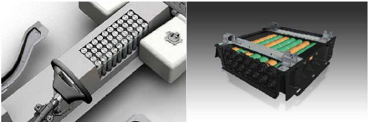
Figure 9 : a) Rendering showing Cylindrical Cells b) Cylindrical cells in a battery pack for Honda Civic Hybrid
