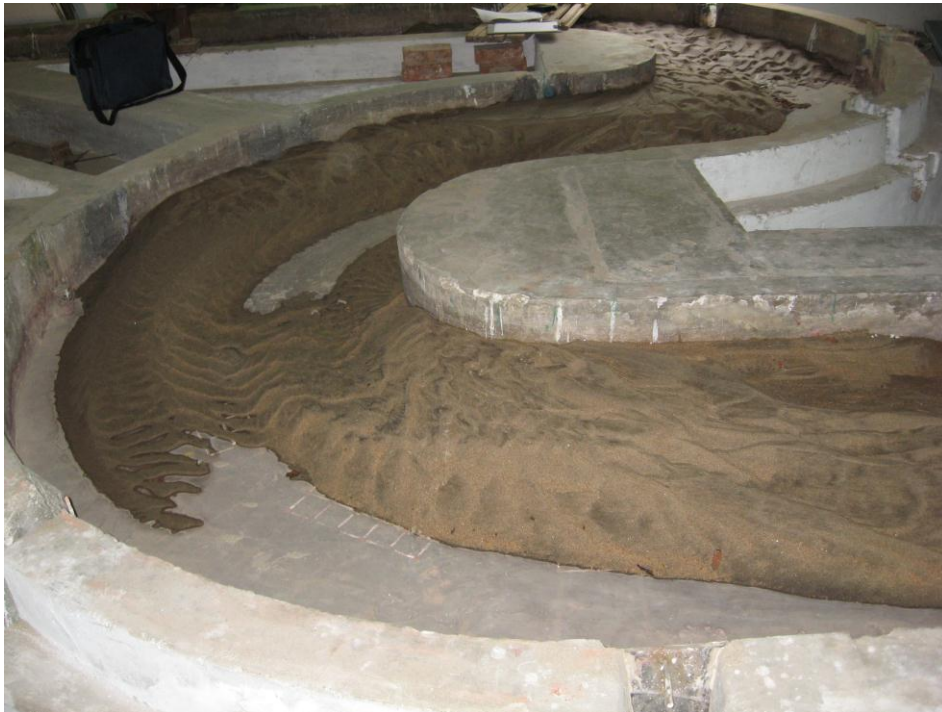
Figure 2: Photograph showing the erosion and deposition taking place in the meandering channel
